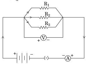
In the circuit given below, the resistors  $R_1$ ,  $R_2$  and  $R_3$  have the values 10  $\Omega$ , 20  $\Omega$  and 30  $\Omega$  respectively, which have been connected to a battery of 12 V. Calculate
